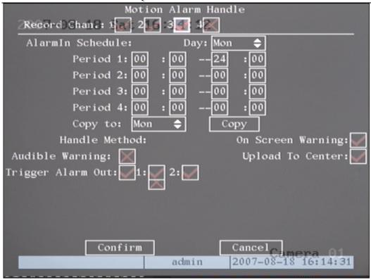
Fig 5.18 Motion alarm handle setup
